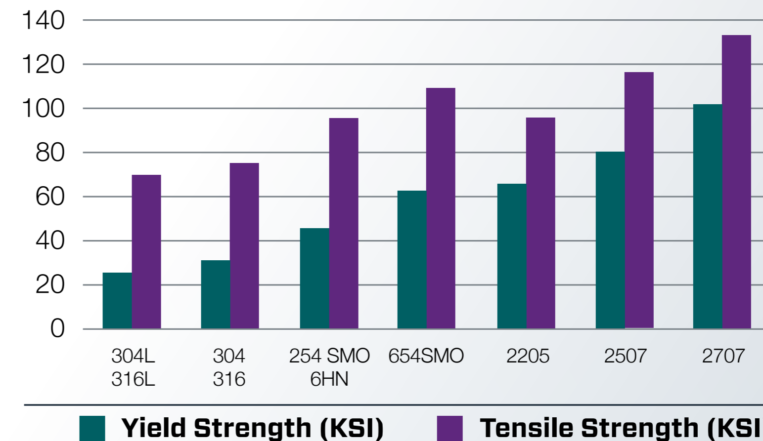
The mechanical properties of alloy 2507 make it a very good choice for high-pressure offshore applications and subsea systems where corrosion, fluid flow, and weight are of concern.
